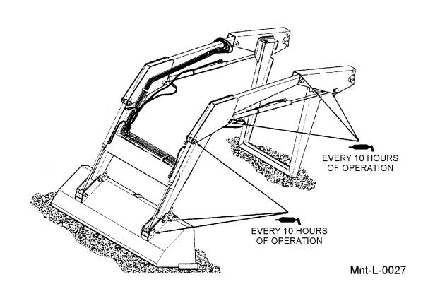
Lubricate all grease fittings: one at each end of lift boom arms and one at rod and base ends of each lift and bucket cylinders.
